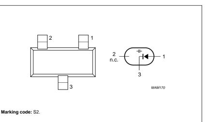
Fig.1 Simplified outline (SOT23), pin configuration and symbol.
